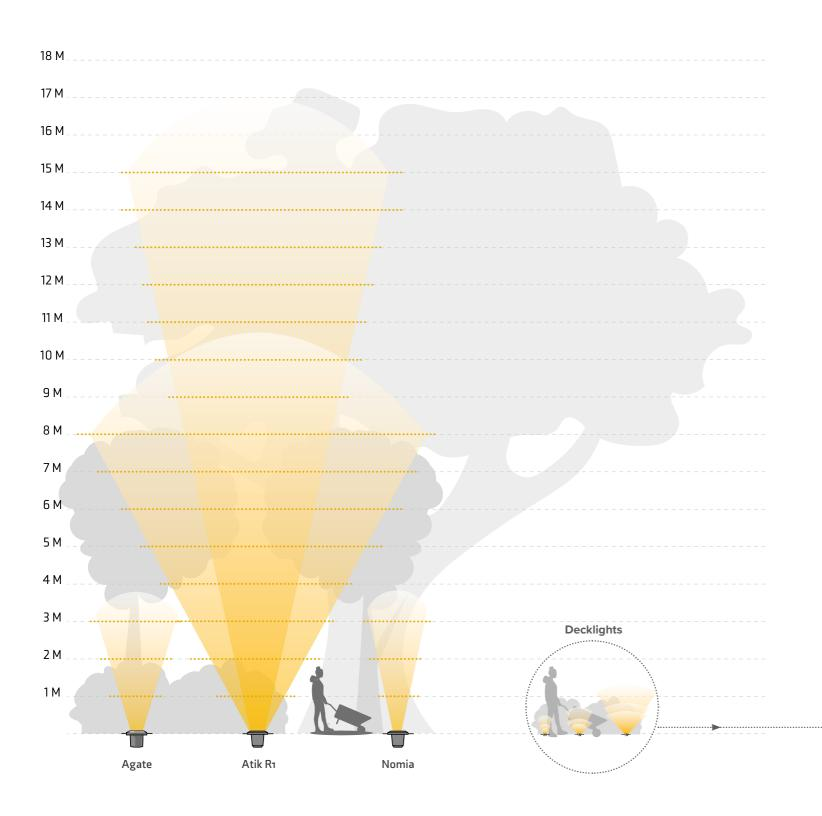
Decklights are most commonly used as orientation lights. In the image below you can easily compare the different decklights and select the right one.
