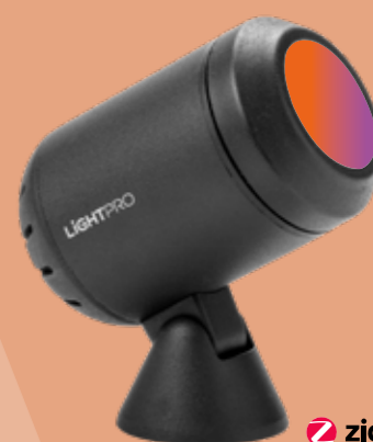
Castor Smart (Zigbee) (200N) Aluminium - Anthracite LED 5 W RGB 280 lm 95 x 60 x 120 mm (H x W x D)
