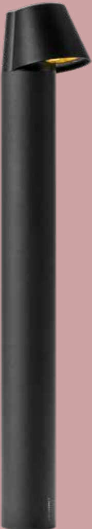
Oberon DL (192P) Aluminium - Anthracite LED 9 W 3.000 K 75 - 750 lm 600 x 93 x 110 mm (H x W x D)
