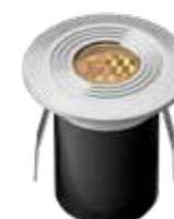
Onyx 30 RS (240D) Stainless steel 316 LED 0,5 W 2.700 K 4 lm 59 x 45 mm (H x Ø) Drillhole 30 mm
