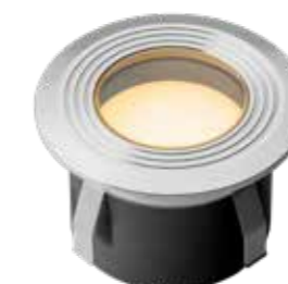
Onyx 60 RS (242D) Stainless steel 316 LED 1 W 2.700 K 23 lm 59 x 75 mm (H x Ø) Drillhole 60 mm
